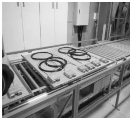
Fig. 15 Irradiation pallet on roller conveyer
