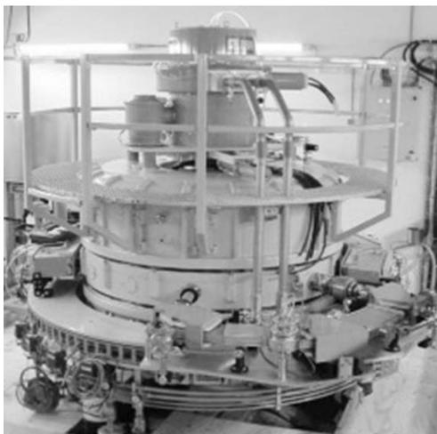
Fig. 13 Rhodotron that is used for radiation-resistant experiment (max. current: 10 mA, max. energy: 10 MeV)
