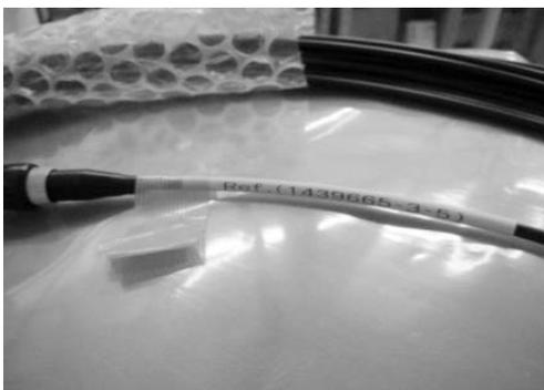
Fig. 14 Single-mode optical fiber irradiated by  $\gamma$ -ray and electron (upper). FC connector (lower)
