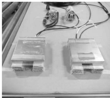
Fig. 16 Two motors and protection covers
