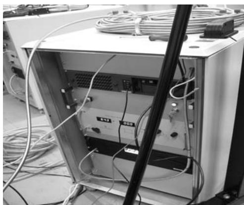
Fig. 18 FO1000 single-mode fiber laser oscillator supplied by Mitsui Bussan Electronics, and 40-m long quartz optical fiber
