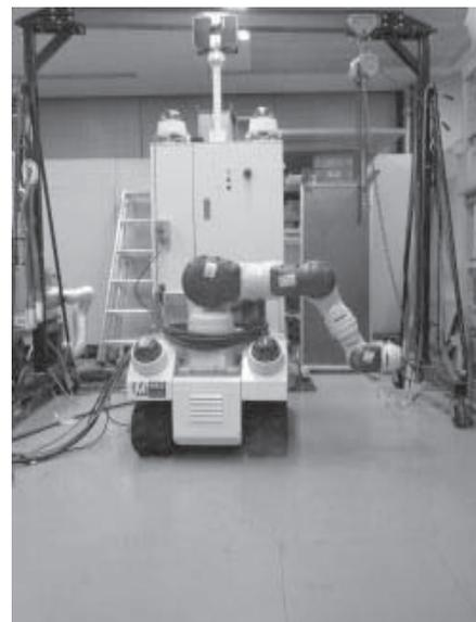
Fig. 10 World's first remote controlled laser decontamination Robot in WERC
